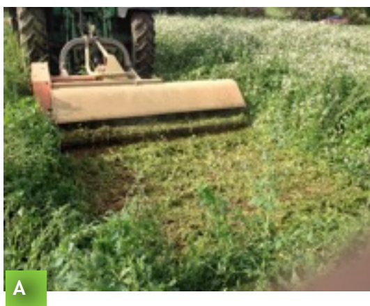
Fig. 13. Incorporation of biofumigants showing A = maceration using a flail mower, B= incorporation with a rotovator, C = incorporation and soil sealing with a spader and D= soil sealing with Cambridge rolls
